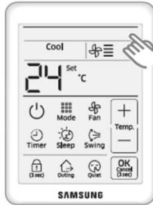
Press and hold the hidden button on the upper right corner of the display
