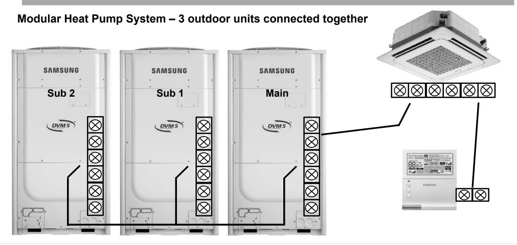
**Heat Pump System & Centralized Control**
