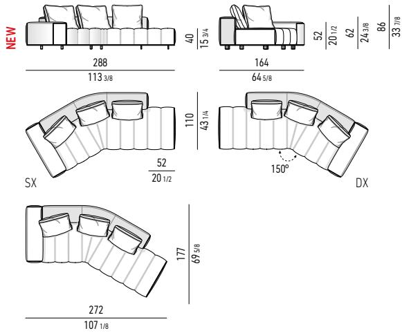
ELEMENTI CENTRALI INCLINATI | INCLINED CENTRAL ELEMENTS
