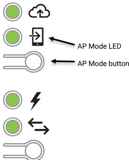
2. The AP Mode LED
