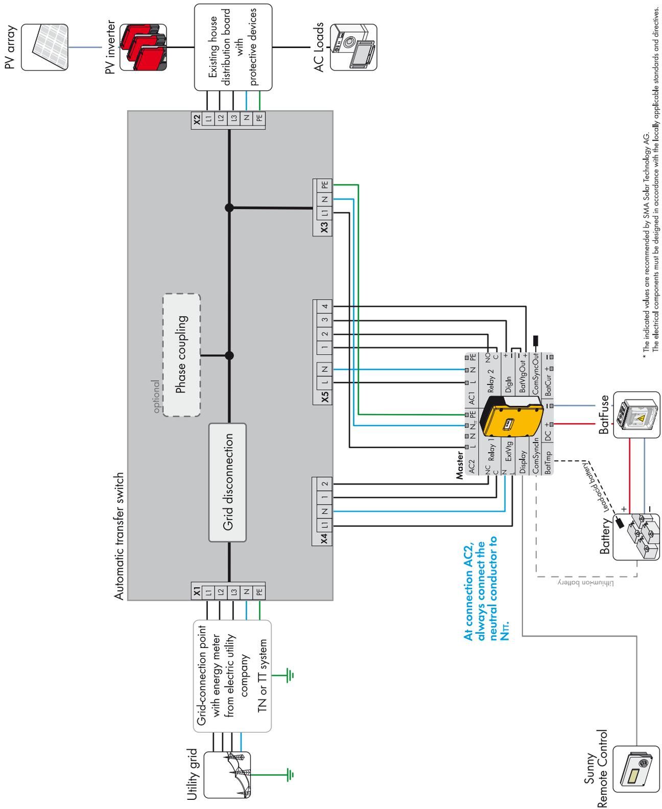
Figure 12: Connection of the automatic transfer switch without all-pole disconnection (e. g. for Australia)
