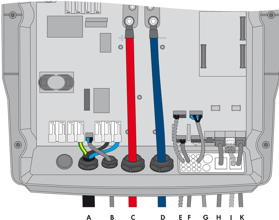
Figure 16: Connecting the master
