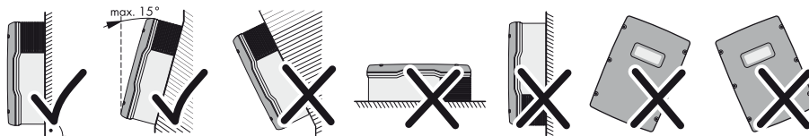
Figure 5: Permissible and impermissible mounting positions
