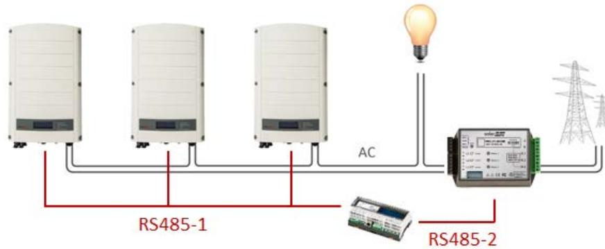
Figure 6: Multi-inverter connection with CCG, RS485 meter and RS485 communications
