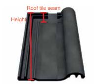
The upper edge to the roof tile. The arm of the roof hook must present a clearance of at least 5mm to avoid it resting upon the roof tiles. Underlayment spacers can be used to achieve the universal height required, depending on the thickness of roof rafters.
