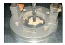
• Drill the metal sheet with a sufficient diameter (for example 30mm), then pre-drill a whole for the hanger bolt with 0.7 x diameter (about 8.5mm).
