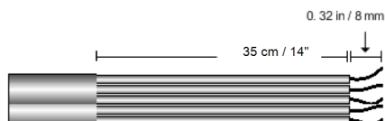
Figure 33: Insulation stripping – AC
