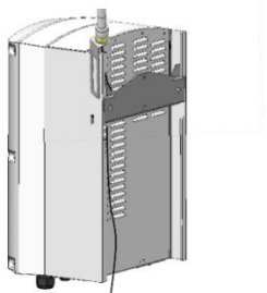
Figure 3: Routing the antenna cable (Three phase inverter)
