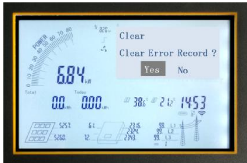
Figure 8 Clear fault interface
