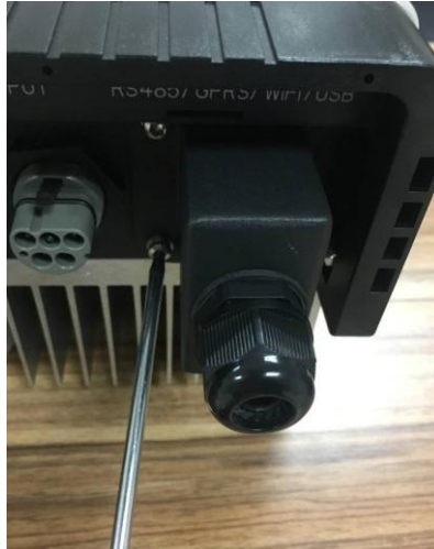
Fig. Dismantle the communication box
