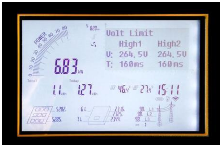
Figure 19 set Over voltage and frequency limit interface
