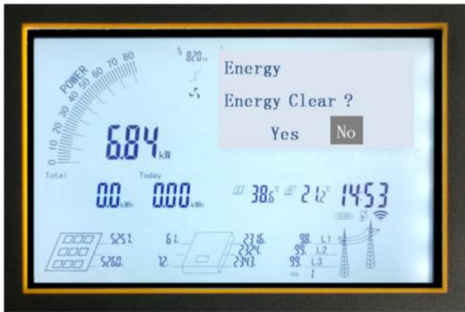
Figure16 Clear generating capacity interface
