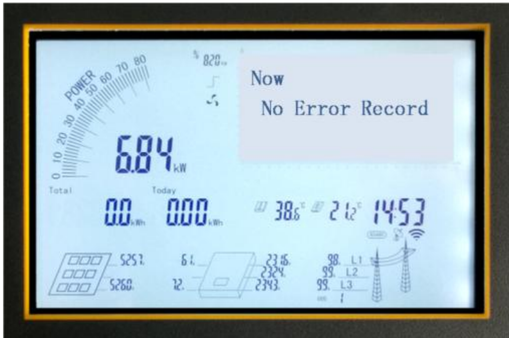
Figure 9 Current fault record interface
