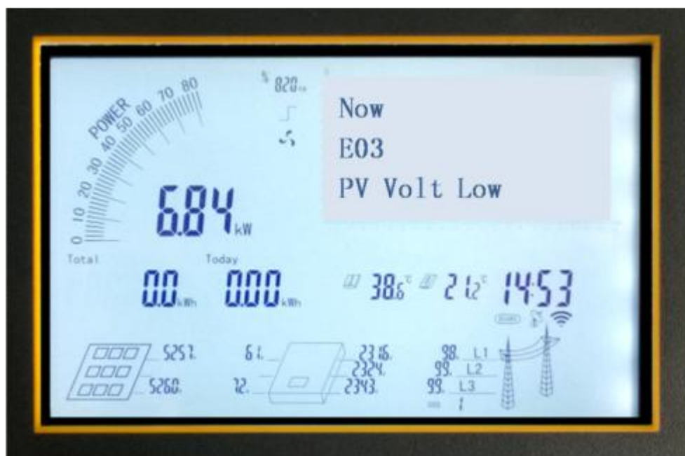
Figure 10 Current fault record interface
