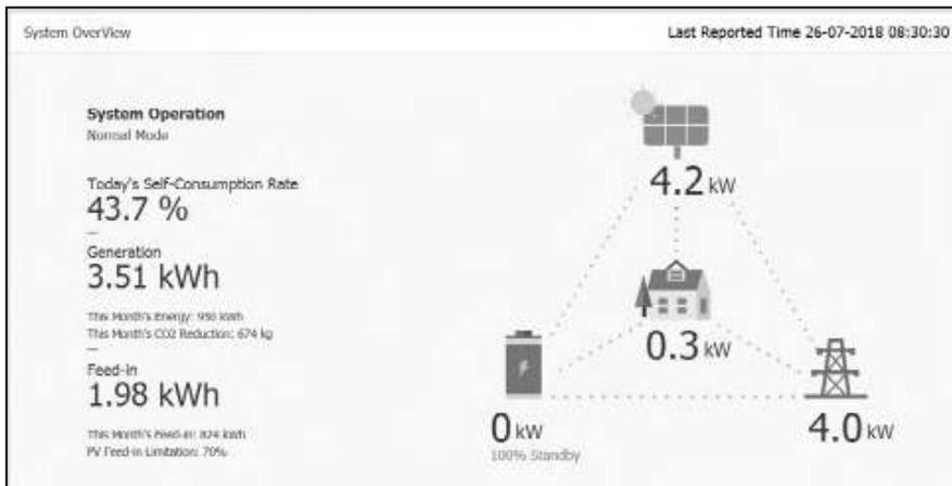
Displays the status of the system. This page provides you with system information such as current power generated from PV, power purchased from grid, power charged/discharged from the battery. ALL the information is renewed every 10 seconds.
