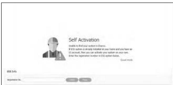
You can see the screen on the left when the registration is in incomplete status. Input the registration number printed in the label attached outside of the PCS and select [Check] to complete the registration and activation.
