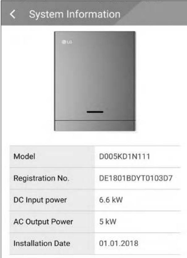
Displays system information of this ESS. You can check information on PCS, battery and network status. Scroll up or down to display next or previous information.
