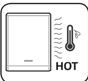
The right side of the installed PCS can be hot by the heat from air outlet. Do not place any object near air outlet.
