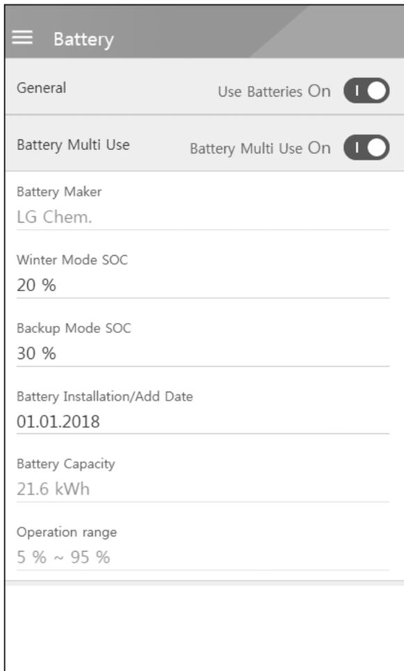
[Battery maker], [Operating range], [Winter Mode SOC] [Battery Installation Date] and [Battery Capacity] can be set manually.
