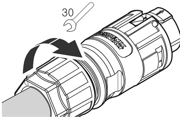
Assemble the rubber seal into the housing and fasten the cable gland to the housing using 30 mm wrench. (4.5 N.m)
