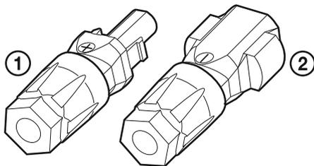
Check the components of battery cable plugs which is supplied in the product package.
