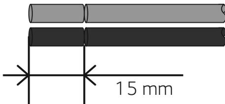
Strip 15 mm off the both + and - battery wires as shown in the figure.
