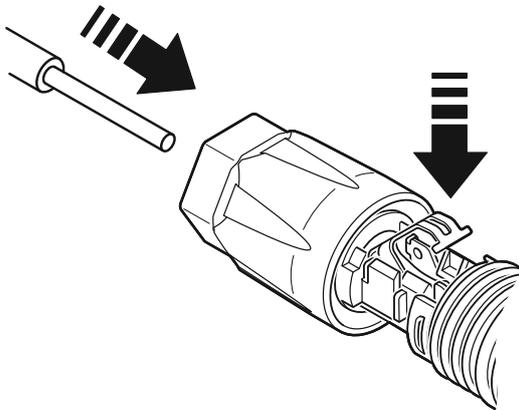
Carefully insert the stripped wires to the corresponding cable connector. The wire ends have to be visible in the spring.
