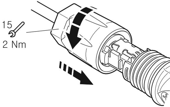
Push the insert into the sleeve and fasten the cable gland to the housing using 15 mm wrench. (2 N.m)
