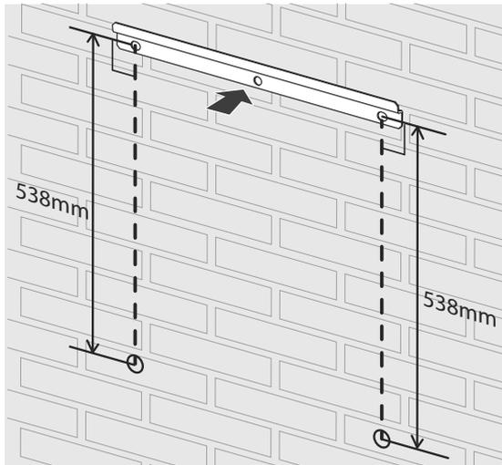
Place the wall bracket on a wall where meets every installation conditions and clearance.
