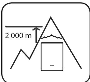
This product must not be installed or used at altitudes above 2 000 m.
