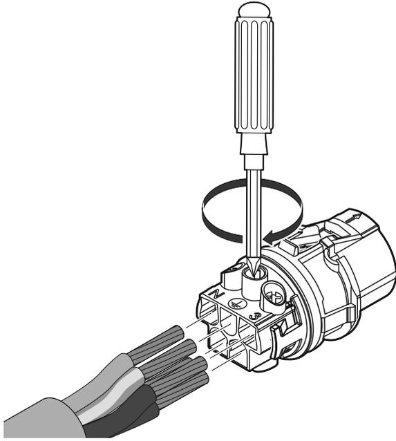
Connect the wires to the corresponding wire holes on the contact carriers.
