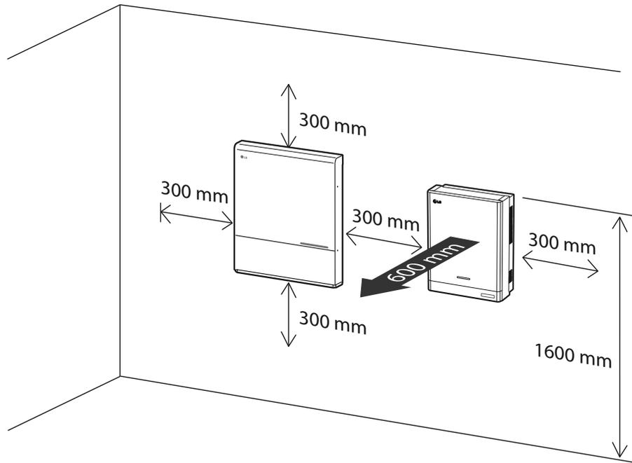
This product must be installed with clearance at the left, right, top, bottom and front of the product as shown in the figure.
