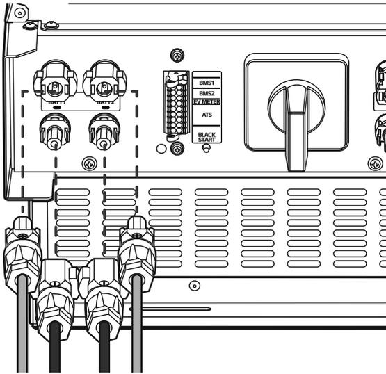
Connect the both battery cable plugs to the battery DC cable connectors at the bottom of the product.
