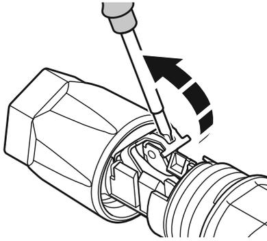
Open the spring using a screwdriver
