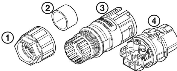
Check the components of grid cable plug which is supplied in the product package.
