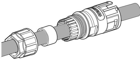
Pass the AC cable through the cable gland, rubber seal and housing as shown in the figure.
