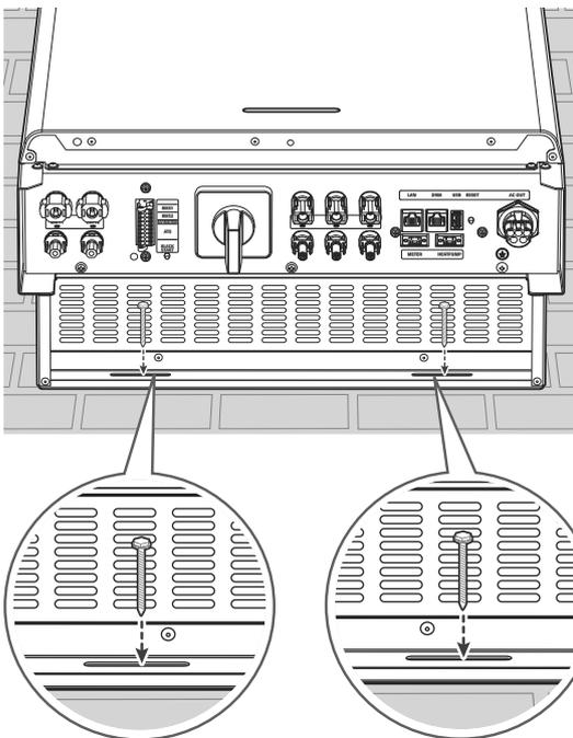
Drill holes on the screw hole positions and fix the product to the wall with screws and anchors.
