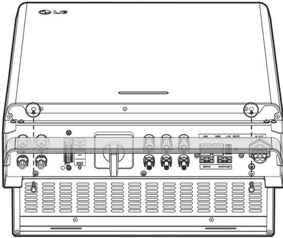
After finishing every electrical connections, assemble the supplied lower cover and fix the screws as shown in the figure.
