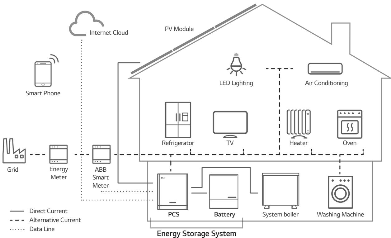
The electricity generated from a PV array can be stored to the connected battery or sold to energy supply companies.
