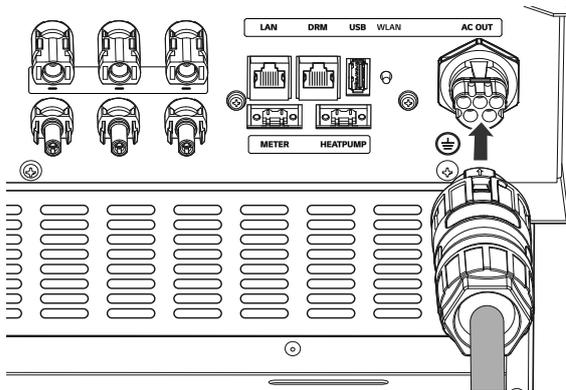
Connect the AC cable plug to the AC grid cable connector at the bottom of the product.
