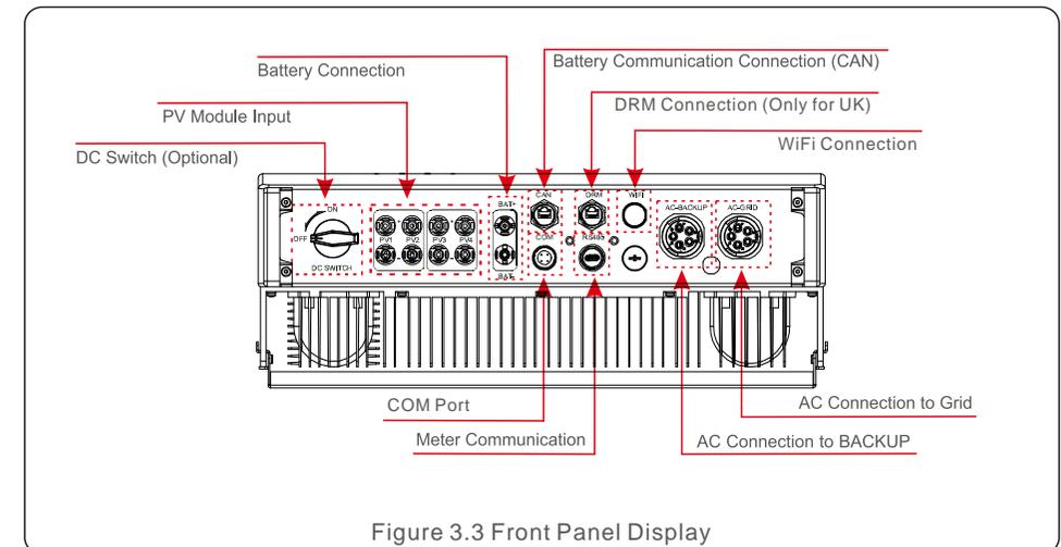
Figure 3.3 Front Panel Display
