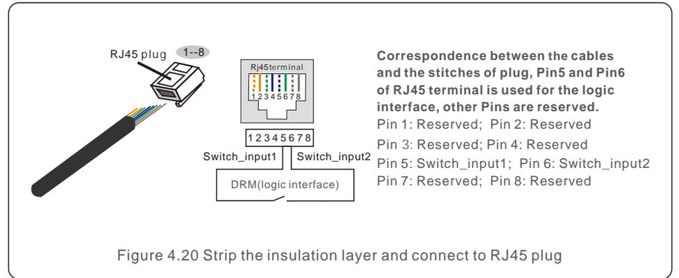
3. Connect RJ45 to DRM (logic interface) .
