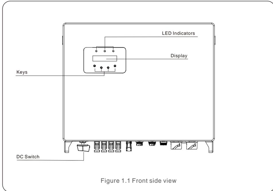
Figure 1.1 Front side view
