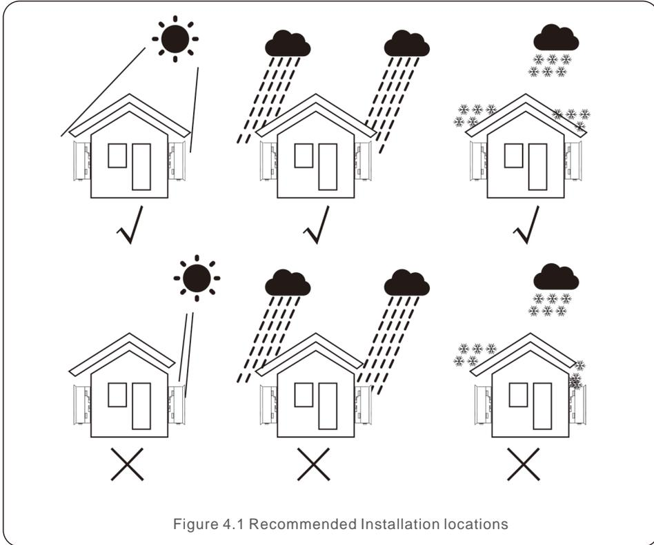
Figure 4.1 Recommended Installation locations
