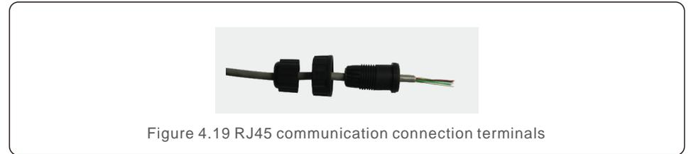
2. Use the network wire stripper to strip the insulation layer of the communication cable. According to the standard line sequence of figure 4.20 connect the wire to the plug of RJ45, and then use a network cable crimping tool to make it tight.
