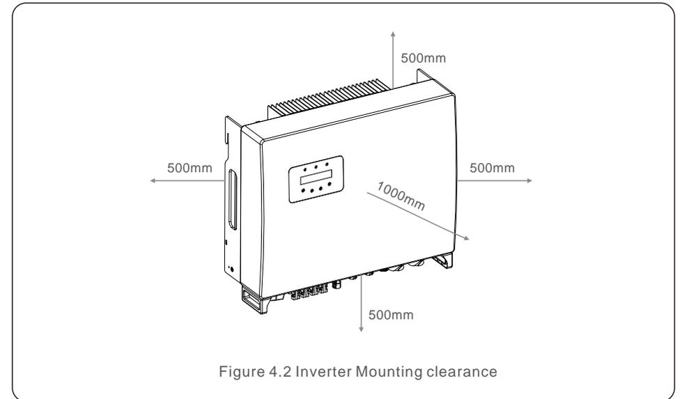
Figure 4.2 Inverter Mounting clearance
