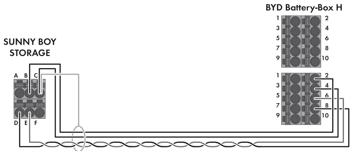
Figure 2: Cabling plan SBS2.5-1VL-10 with Battery-Box H
