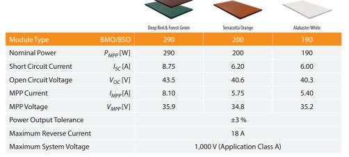
Efficiency at irradiation 200 W/m<sup>2</sup>: 99.3 % of STC efficiency or higher. | Power measurement tolerance: ±3 %.
