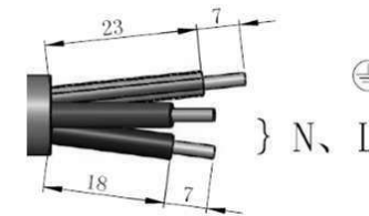
Figure 4.15 Stripped AC Wires
