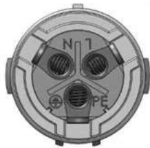
Figure 4.13 AC Grid Terminal Connector Inside
