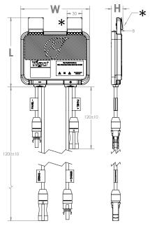
\*Clips can be removed for rack mounting
