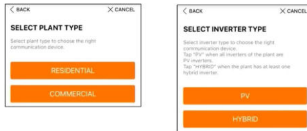
figure 7-3 Selecting Plant/Inverter Type
