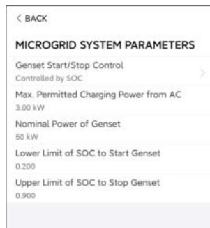
figure 8-29 MicroGrid System Parameters
