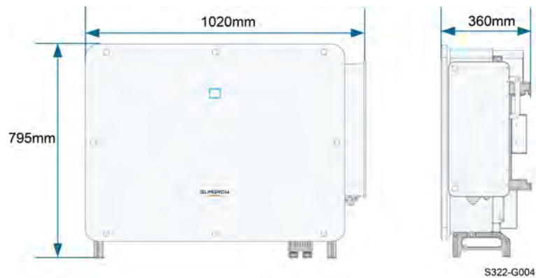
figure 2-3 Product Dimensions(in mm)
