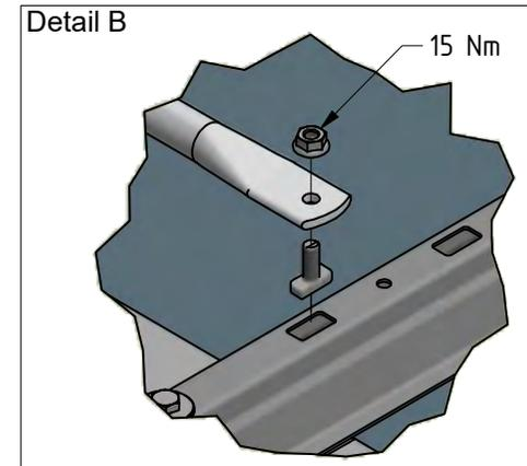
Mount the push rods on the roof carriers to connect the two rows.
