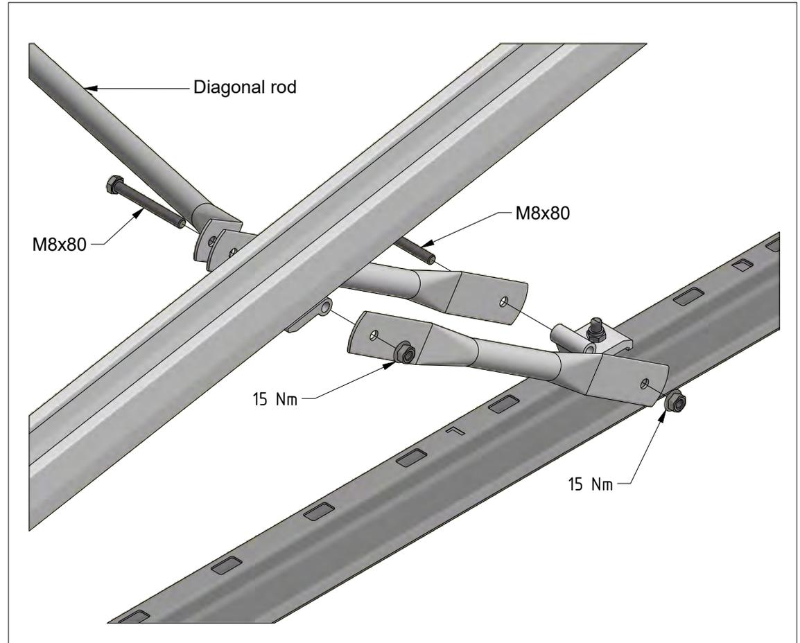
Mount the push rods to the aluminium profile and the roof carriers.
