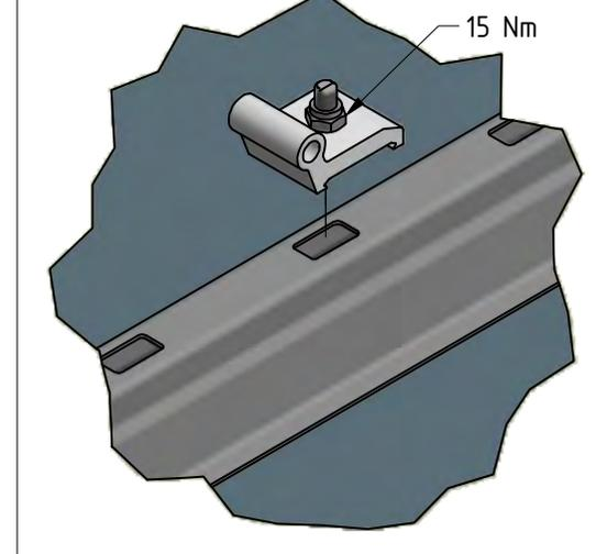
Mount the connector pieces to the roof carriers. Make sure they are placed as shown in the drawing.
