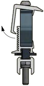
Take the end clamp out of its slot for an easier assembly.
