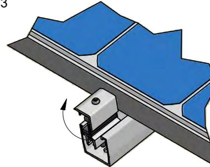
The end clamp can only be turned clockwise, so make sure the end clamp is placed the right way.
