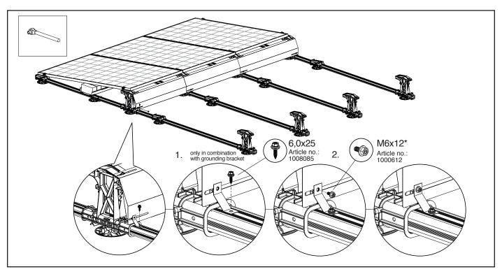
\*Esdec tested and approved the M6 x 12 metric screw for fixing the rear wind deflector to the high plastic base.
