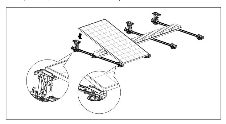
3. Place the end clamps on the edge of the solar panel and position them at the mounting holes in the high and low bases. Screw in the end clamp with the mounting screw into the mounting hole.
