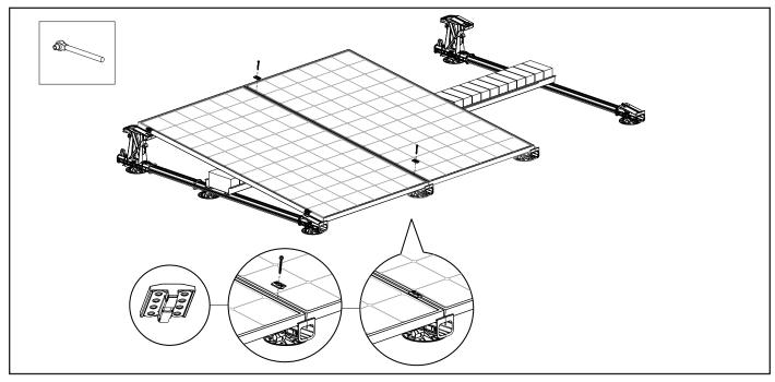
Place the last solar panel of the row on the base elements so that it lies between the upright lugs.
