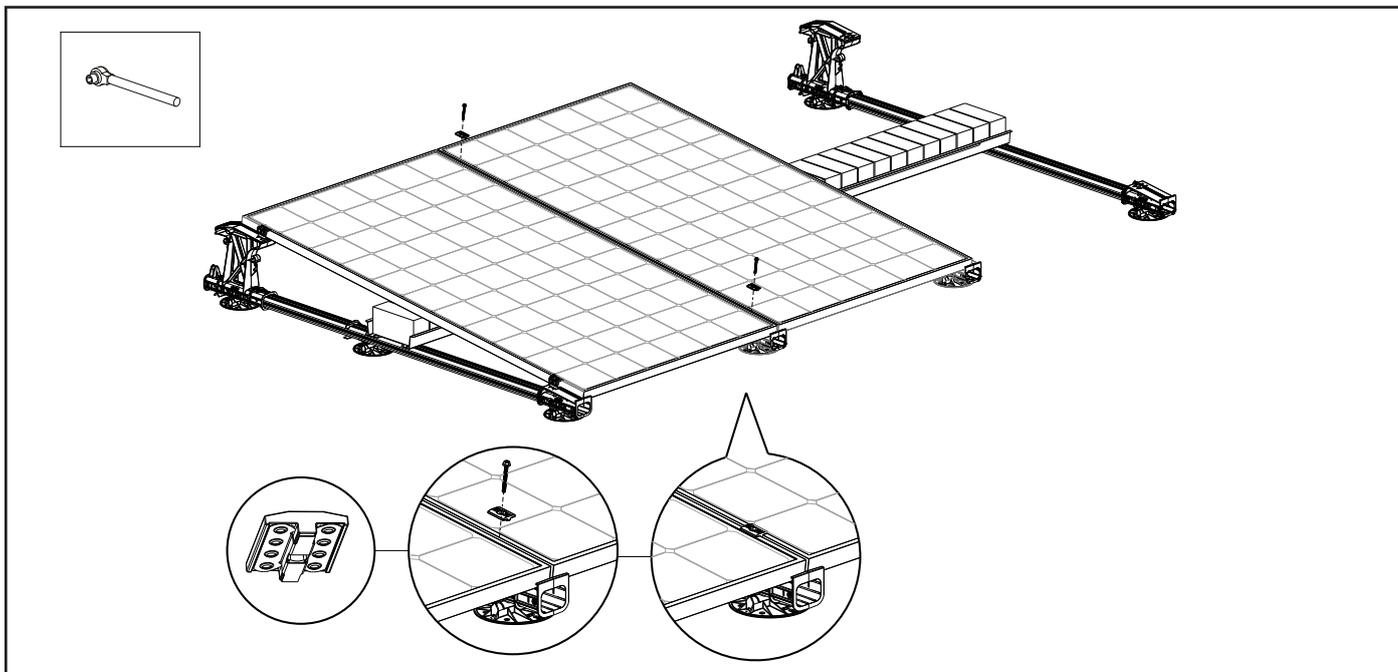
Place the last solar panel of the row on the base elements so that it lies between the upright lugs.
