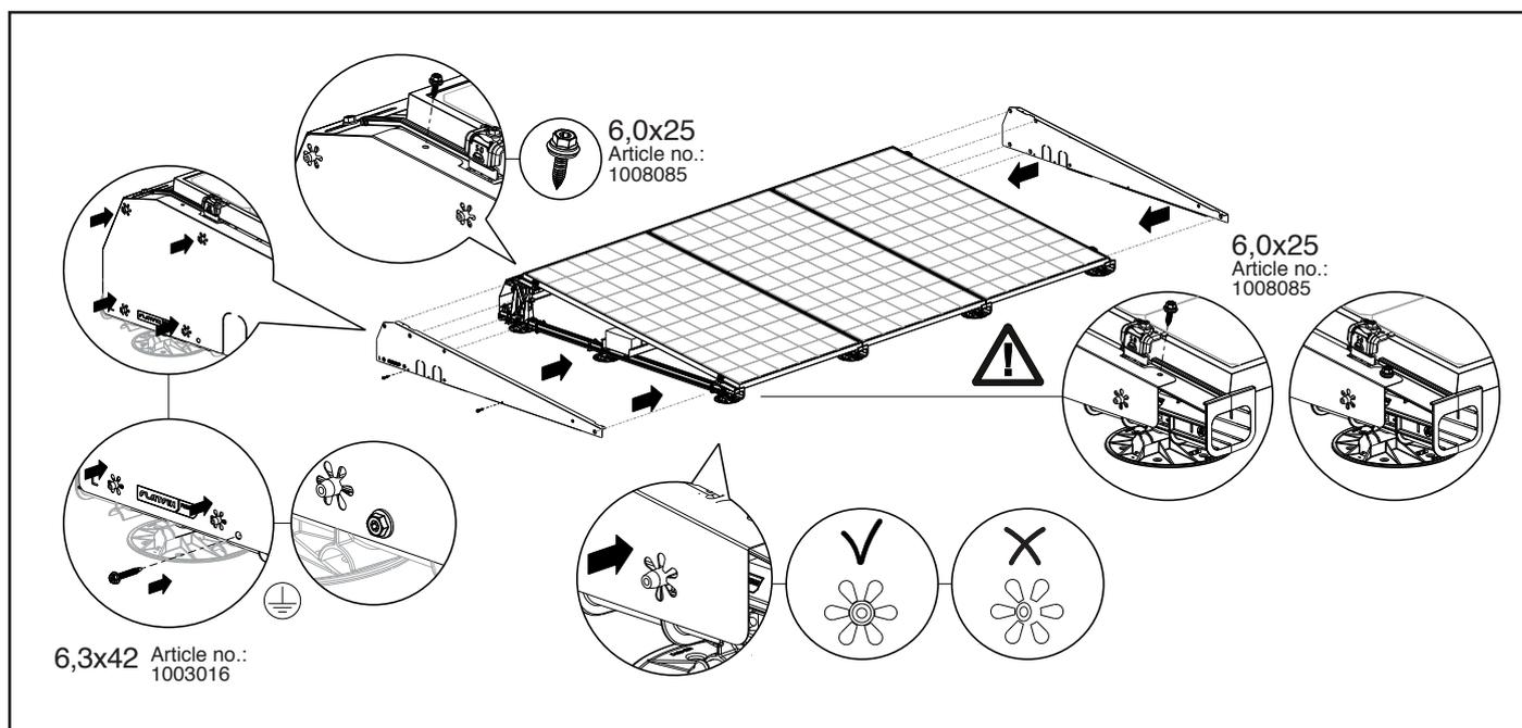
You can now mount the 2<sup>nd</sup> row of solar panels. To do this, follow the installation steps in sections 6.8 to 6.18. The panel field is now ready!
