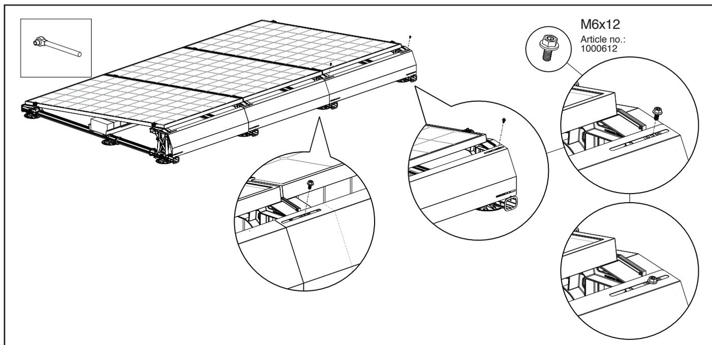
Attach the wind deflectors (on lower sides) to the high bases by placing the mounting screw M6x12 in the slots of the wind deflector and screw it into the mounting holes of the high bases. **NOTE!** The maximum tightening torque of the screw connections is 2 Nm. Make sure that the mounting screws do not slip in the base. Refer to your tool manual to set it to the correct torque.
