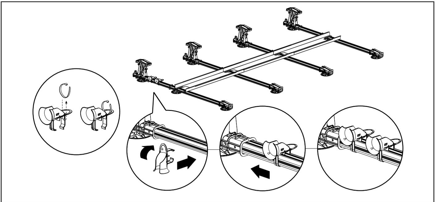
1. Feed all (+) cables through the 1<sup>st</sup> cable exit guide and all (-) cables through the 2<sup>nd</sup> cable exit guide. Secure the cables in the cable exit guides using cable ties to prevent cable play.
