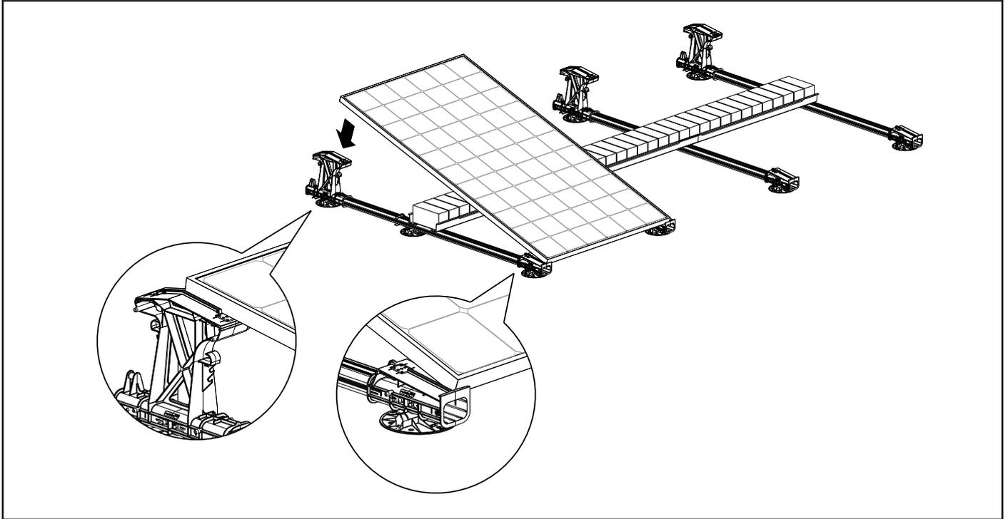
3. Place the end clamps on the edge of the solar panel and position them at the mounting holes in the high and low bases. Screw in the end clamp with the mounting screw into the mounting hole.
