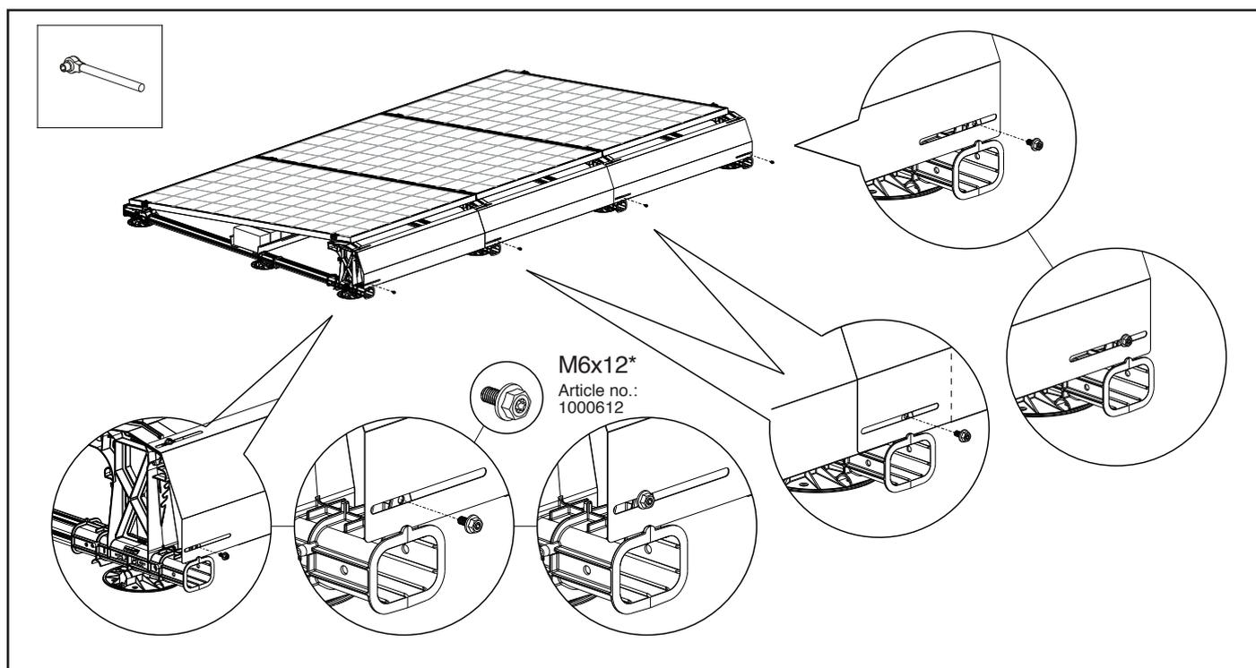
*\*Esdec tested and approved the M6 x 12 metric screw for fixing the rear wind deflector to the high plastic base.*
