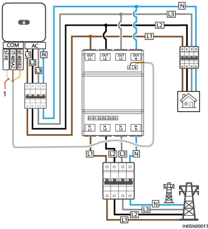
**Figure 5-27** Three-phase, three-wire direct connection (SmartLogger networking)
