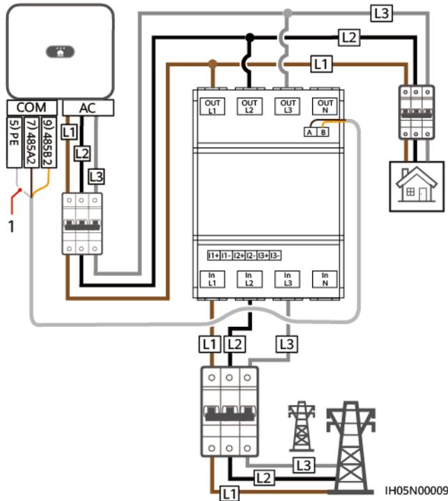
**Figure 5-26** Three-phase, four-wire direct connection (Smart Dongle networking)
