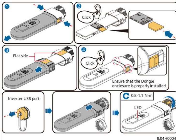
**Figure 5-49** Installing anti-theft components for the Smart Dongle
