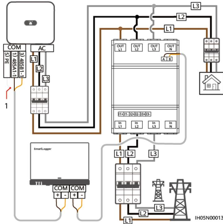
**Figure 5-28** Three-phase, four-wire direct connection (SmartLogger networking)
