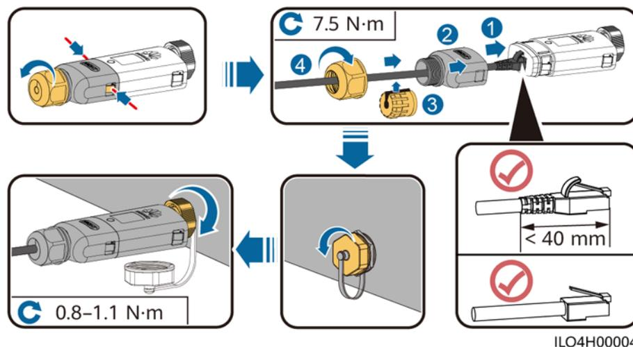
**Figure 5-47** Installing anti-theft components for the Smart Dongle
