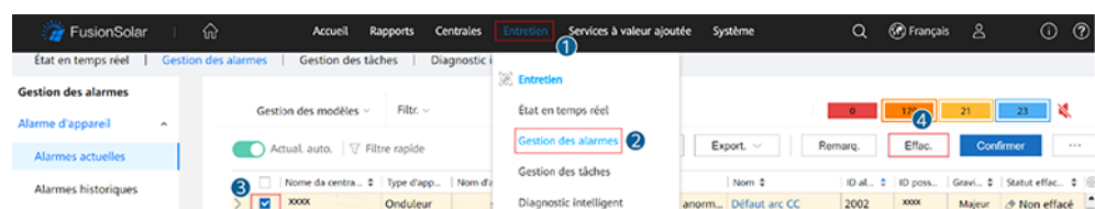
Figure 7-8 Effacement des alarmes
