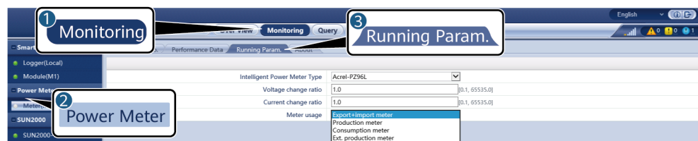
Figure 6-33 Setting power meter parameters
