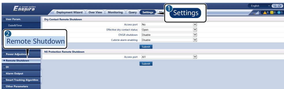
Figure 6-63 Dry contact remote shutdown
