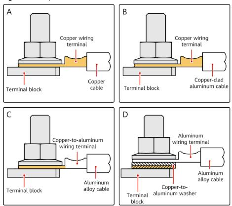
Figure 5-2 Requirements on an OT or DT terminal
