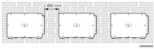
Figure 4-5 Triangle installation mode (recommended)
