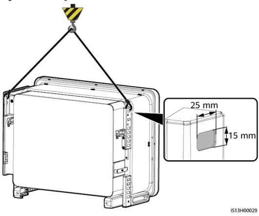
Figure 4-14 Hoisting the inverter
