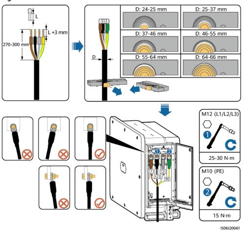
Figure 5-12 Cable connection
