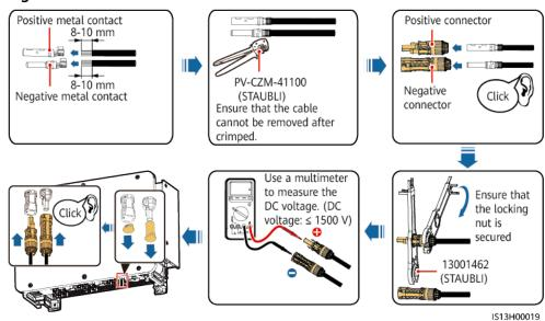
Figure 5-17 Connector connection
