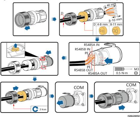
Figure 5-21 Cable connection (4–8 mm two-hole rubber plug)
