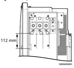
Figure 5-10 Specification of the Rubber Baffle Plate
