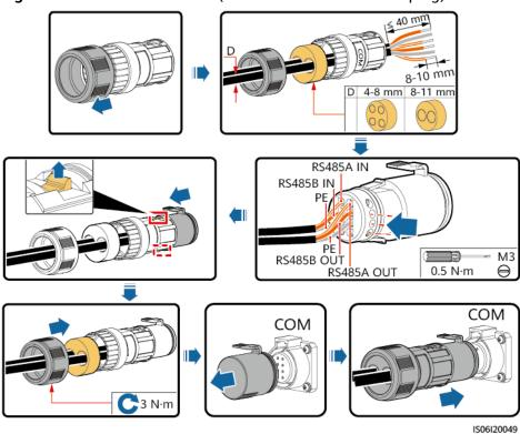
Figure 5-20 Cable connection (4-8 mm four-hole rubber plug)
