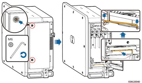
**Step 3** Remove the accessories that are bound in the maintenance compartment for future use.
