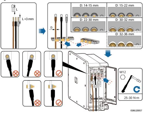
Figure 5-13 Cable connection
