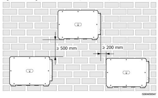
Figure 4-6 Stacked installation mode (not recommended)
