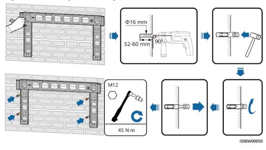
Figure 4-10 Securing the mounting bracket
