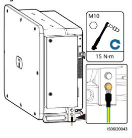
**Figure 5-11** Cable connection
