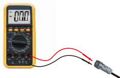
Measure AC voltage and frequency
