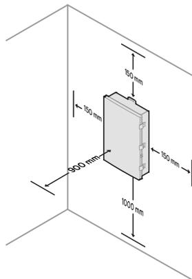
**Dimension de perçage pour l'installation**
