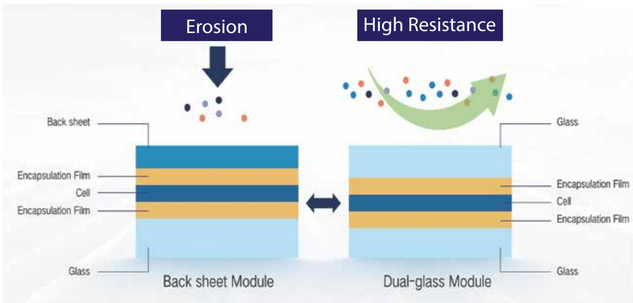
Figure 2. Comparing the structure of backsheet and dual-glass modules
