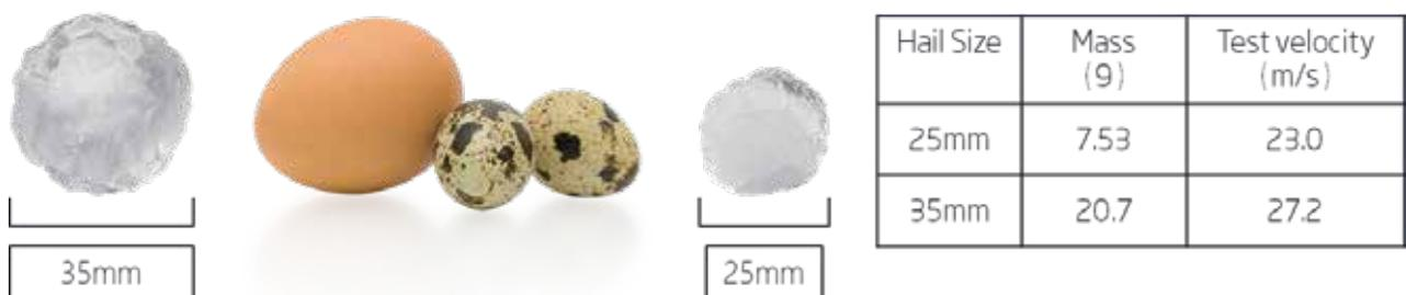
Figure 4. Comparison of hail size and test velocity
