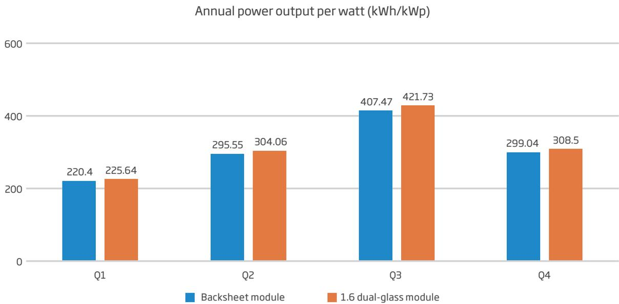
Figure 3. Energy yield at Haikou (backsheet versus 1.6mm dual-glass)
