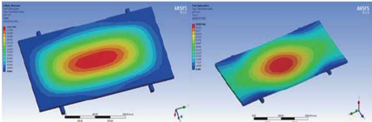
Figure 8. Deformation of backsheet (left) and dual-glass modules (right)
