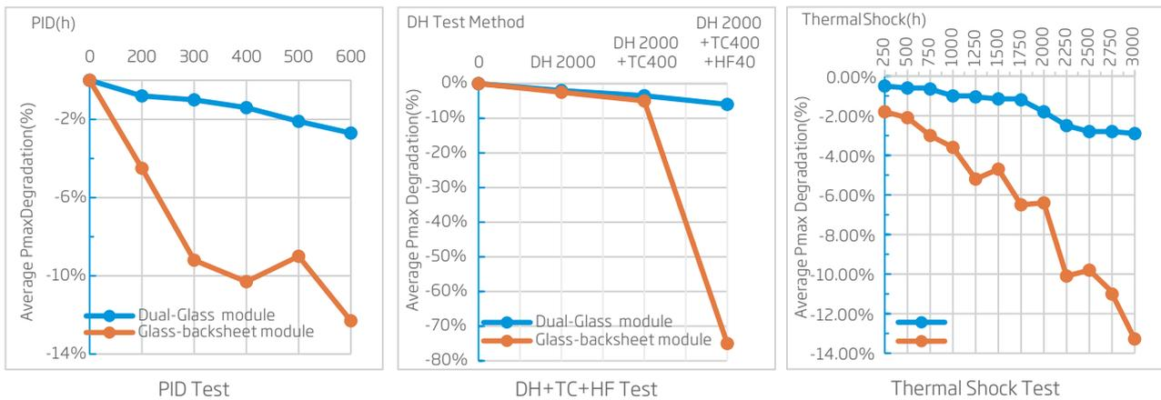
Figure 5. Pmax degradation of dual-glass module and backsheet module after long endurance test
