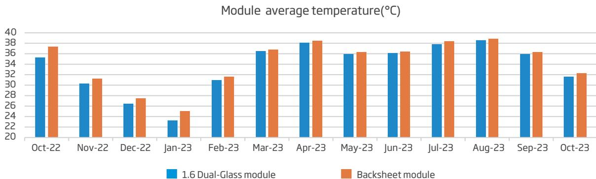
Figure 1. Monthly module temperature(ave.) of dual-glass and backsheet module
