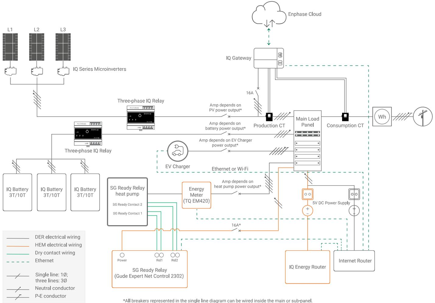
\*All breakers represented in the single line diagram can be wired inside the main or sub-panel.
