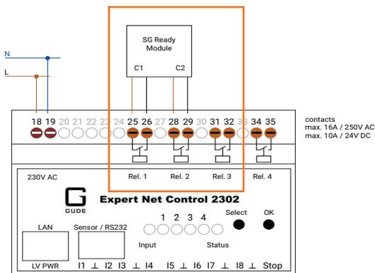
C) **Network connection:** Plug the Ethernet cable coming from the home router or Ethernet switch into the LAN port of the SG Ready Relay as shown in the following figure:
