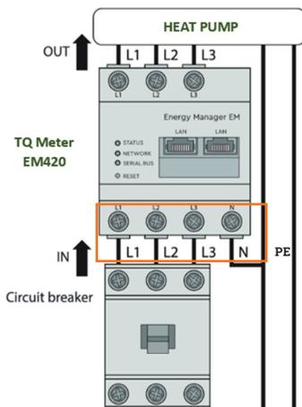
**WARNING:** Make sure the circuit is not energized while working on the electrical connections. Make sure upstream breakers are open and zero voltage is verified using a multimeter.
