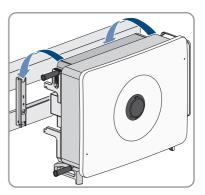
Remove all 4 carrying handles from the threaded holes or remove the eye bolts of the lifting gear and again screw in the sealing screws using a flat-blade screwdriver (4 mm, tightening torque: 2 Nm).
