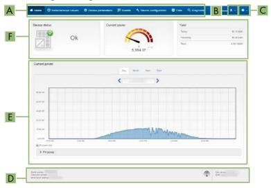
Figure 14: Design of the user interface's home page (example)
