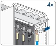
Place the grounding conductor incl. 1 washer and hex nut onto the stud bolt (M8, torque: 20 Nm to 30 Nm) in the middle section. Now tighten it all using a ratchet.
