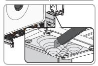
Route the cable through the sealing plate for the AC connection into the device.
