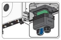
Remove all connection cables from the communication assembly.
