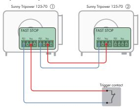
Figure 9: Circuitry overview for connecting a contact for the fast stop and the connection of several inverters
