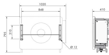
Figure 4: Dimensions of the mounting bracket (dimensions in mm)
