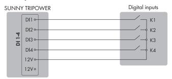
Figure 10: Connection of a remote terminal unit to the digital input DI D1-D4, Vcc of the Sunny Tripower.
