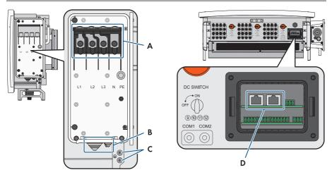
Figure 7: Connection area inside the inverter
