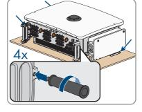
8. Hook the inverter into the mounting bracket.
