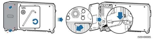
**Step 2** Remove the cover and hang it on the hook of the door.
