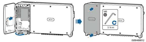
Figure 5-18 Closing the maintenance compartment door
