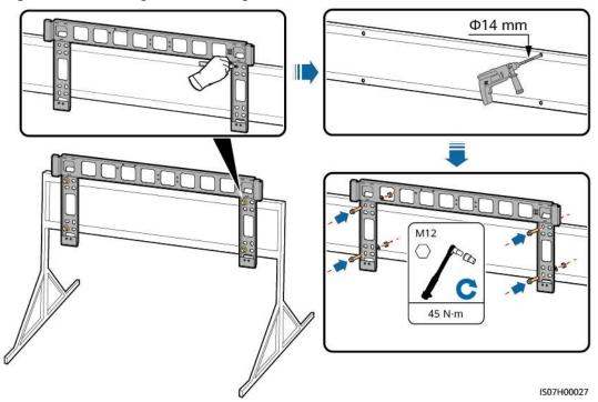
Figure 4-9 Installing the mounting bracket
