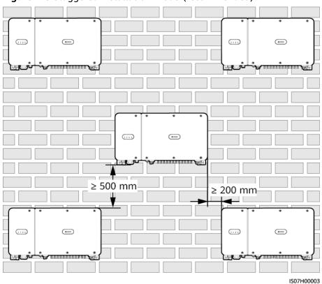
Figure 4-5 Staggered installation mode (recommended)
