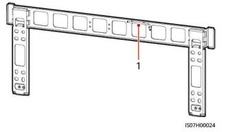
Figure 4-7 Position for binding the security Torx wrench
