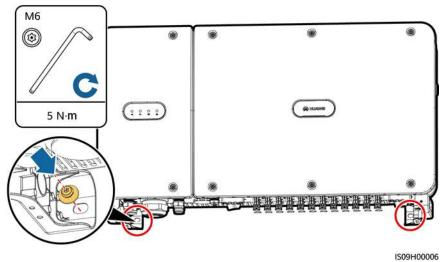
Figure 4-16 Tightening security Torx screws
