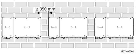
Figure 4-4 Horizontal installation mode (recommended)
