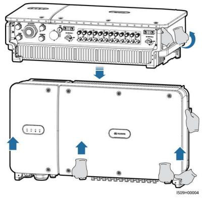
Figure 4-13 Lifting the SUN2000 and keeping it upright
