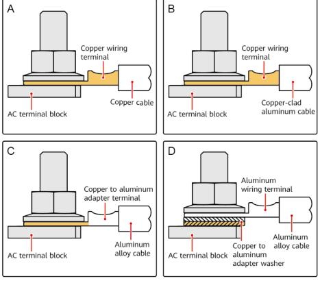
Figure 5-8 Requirements for the OT/DT terminal
