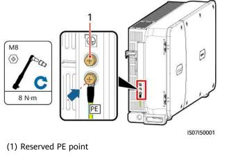
Figure 5-5 Connecting the PE cable to the PE point (on the enclosure shell)
