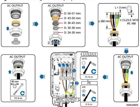
Figure 5-10 Installing the AC output power cable
