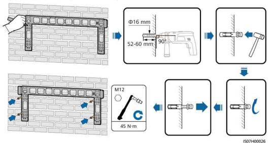
Figure 4-10 Installing the mounting bracket
