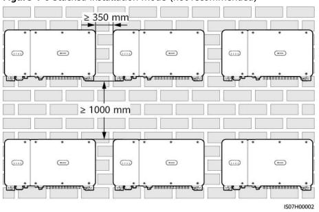
Figure 4-6 Stacked installation mode (not recommended)
