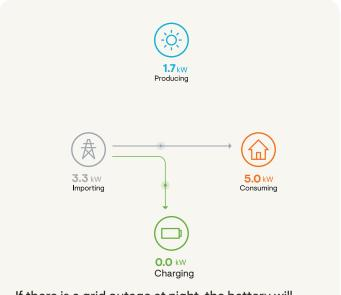
If there is a grid outage at night, the battery will power the backed-up loads. The battery will start charging from the grid once it is back online to restore it to 100% SOC.
