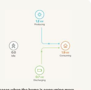
In cases when the home is consuming more power than solar production can provide, the battery starts discharging to meet the power requirement.
