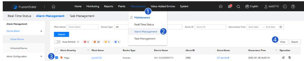
Switch to the owner account with PV plant management rights. On the home page, click the PV plant name to go to the PV plant page, and click **OK** as prompted to clear the alarm.
