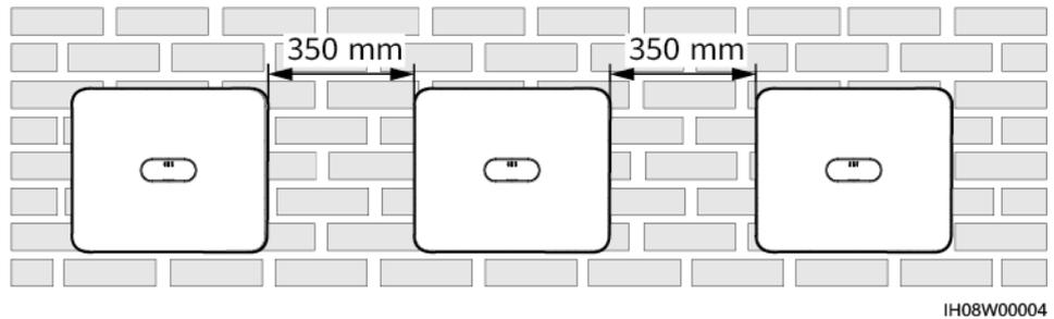
**Figure 4-4** Triangle installation mode (recommended)
