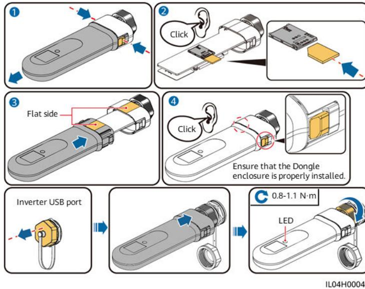
**Figure 5-38** Installing anti-theft components for the Smart Dongle
