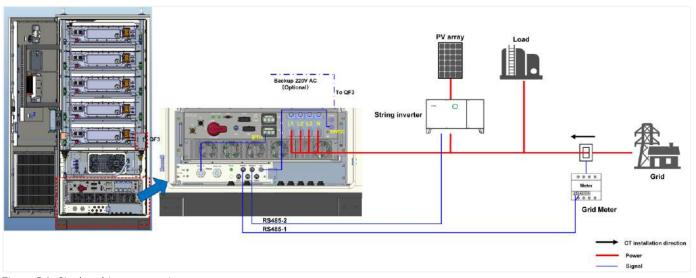
Figure 5.1. Single cabinet connections
