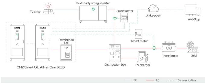
Figure 2.2. System overview of PV-BESS with third-party inverter
