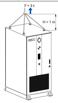
Figure 3.3. Lifting with a crane
