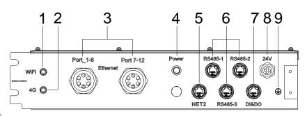
Figure 2.9. EMS unit electrical interfaces
