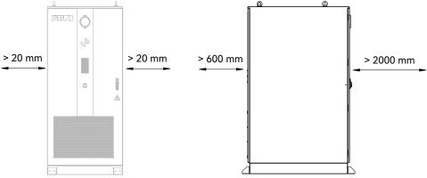
Figure 4.2. Installation space of a single cabinet
