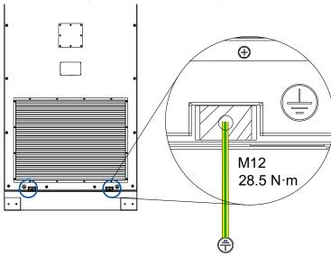
Step 2. Secure the grounding cable to one of the grounding ports at the back bottom of the cabinet.
