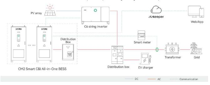
Figure 2.1. System overview of PV-BESS with SAJ inverter
