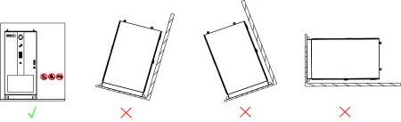
Figure 4.1. Installation position
