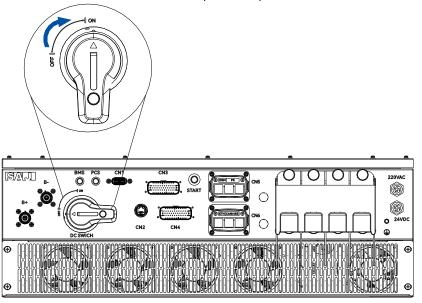
Figure 6.1. Turning on the DC switch
