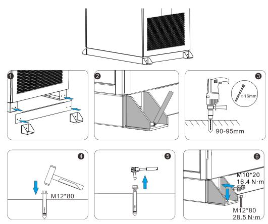
Figure 5.4. Mounting the cabinet
