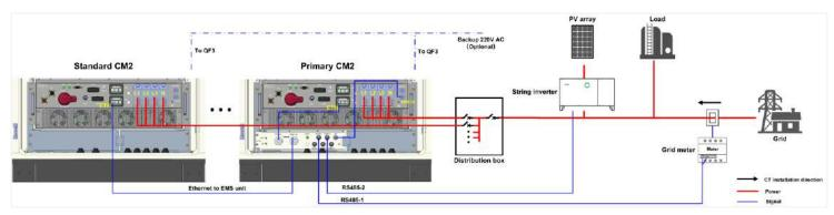
Figure 5.2. Parallel cabinets connections
