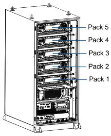
Figure 2.10. Battery pack numbering
