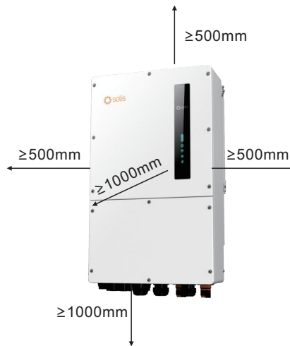
Figure 3.5 Inverter Mounting Clearances
