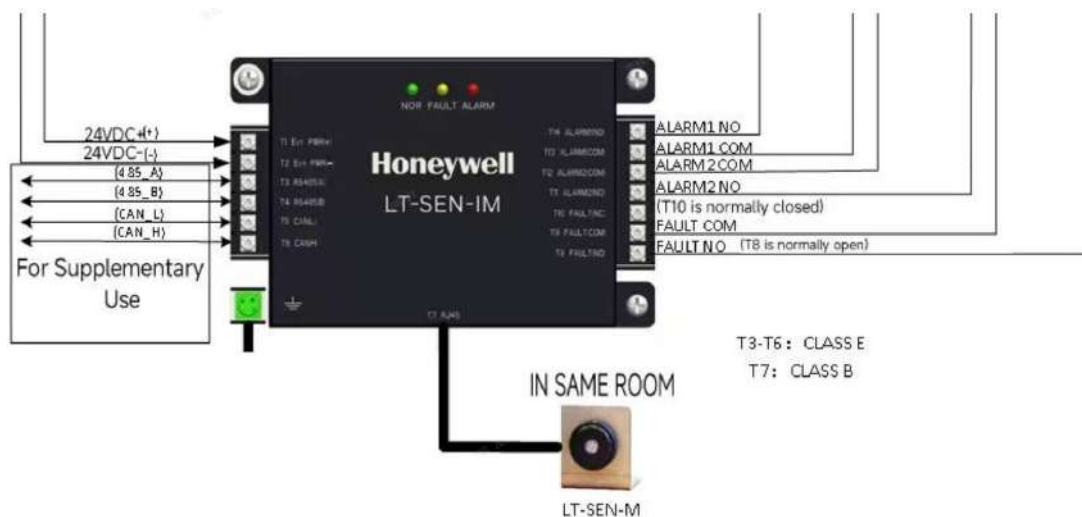
Figure 7-4 Flammable gas detector wiring diagram
