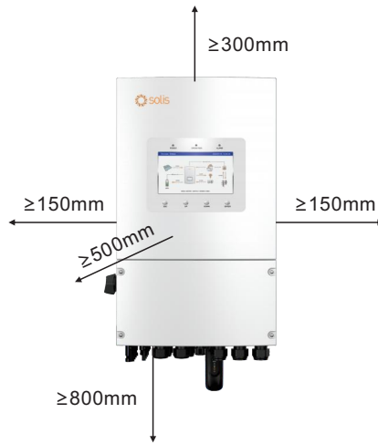
Figure 3.5 Inverter Mounting Clearances
