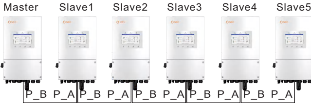
Figure 3.24 Parallel Terminal Connection
