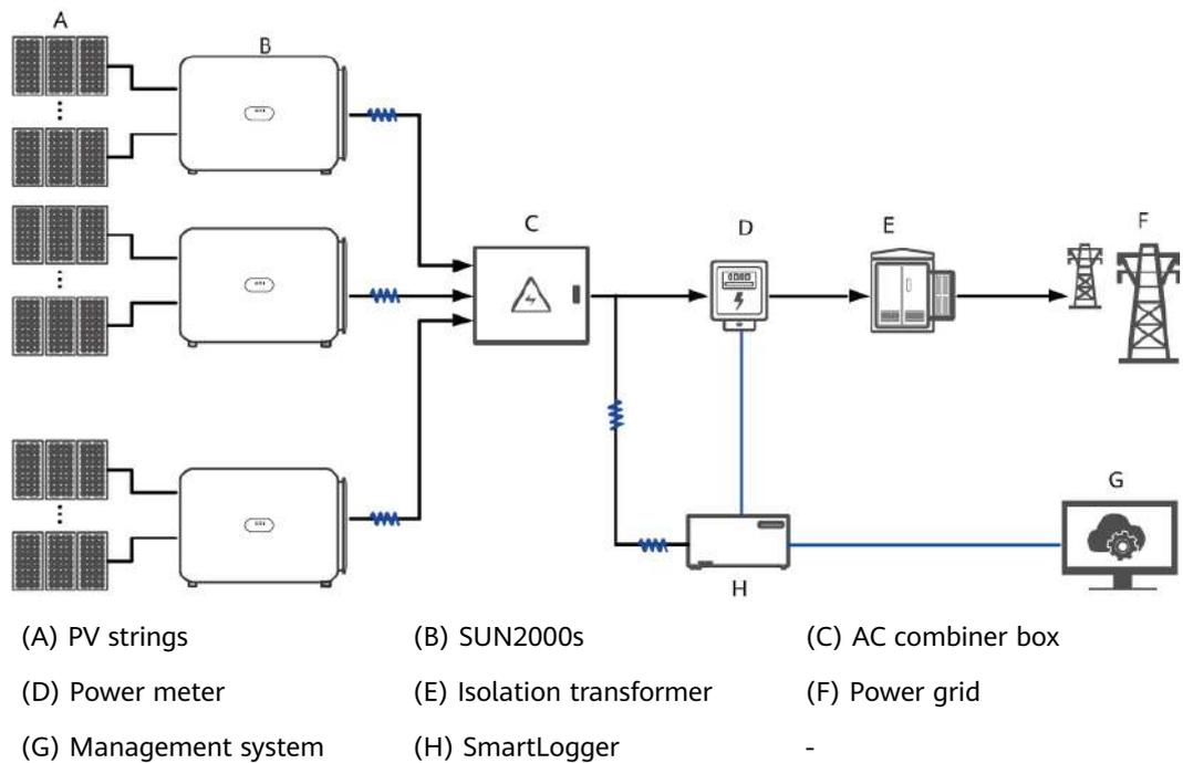
**Figure 2-5** MBUS networking application (Dongle)
