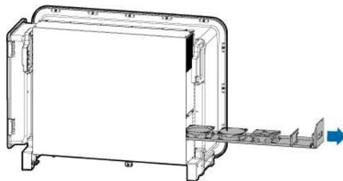
**Step 4** Remove the cable ties from the faulty fan.
