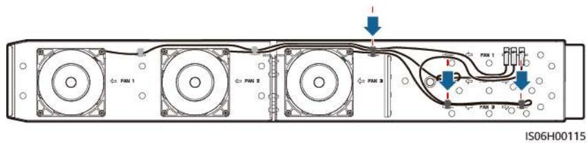
**Step 8** Push in the fan tray until the fan baffle plate is flush with the inverter enclosure.
