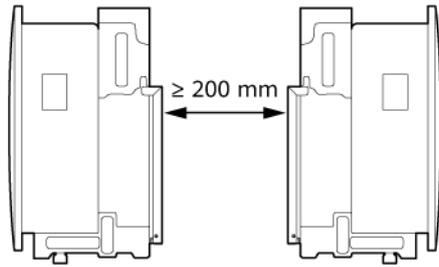
**Figure 4-6** Stacked installation mode (not recommended)
