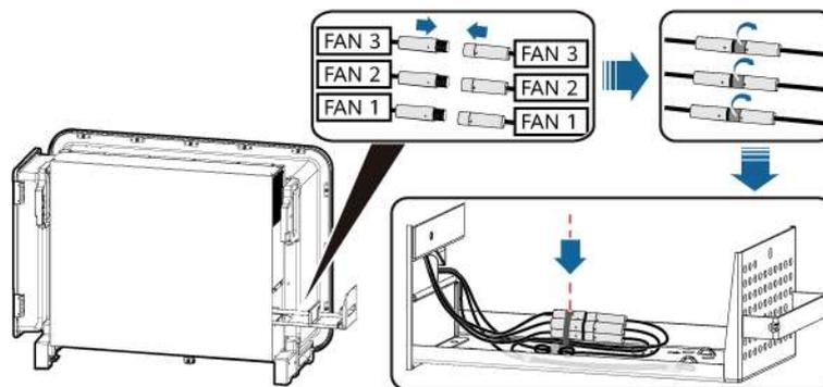
**Step 10** Push in the fan tray completely and tighten the screws.
