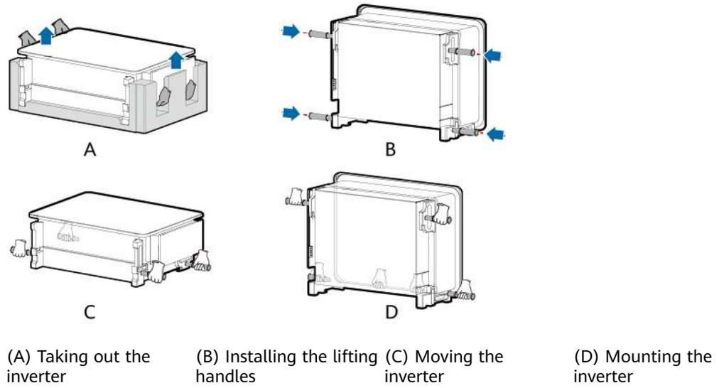
**Figure 4-9** Lifting positions
