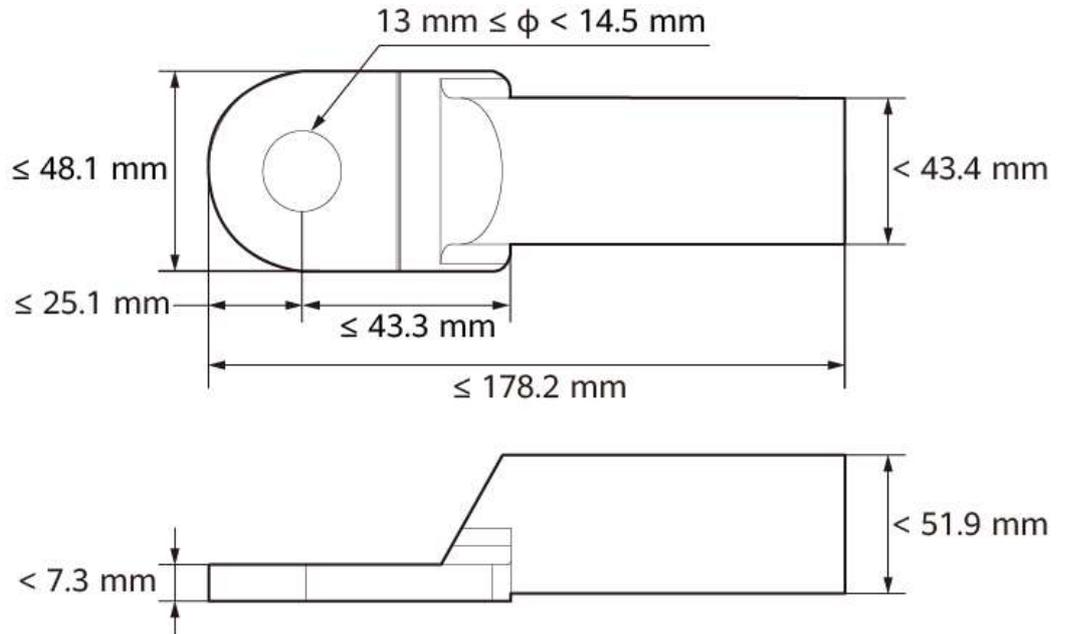
Figure 5-6 Cable connection
