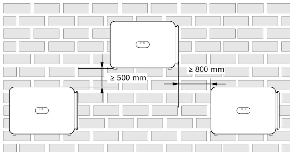
**Figure 4-5** Back-to-back installation mode (recommended)
