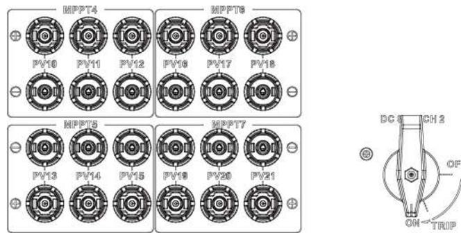
If the DC input terminals are not fully configured with PV strings, evenly distribute the DC input PV strings on each MPPT. For 8 to 20 PV strings, the following DC input terminals are recommended.
