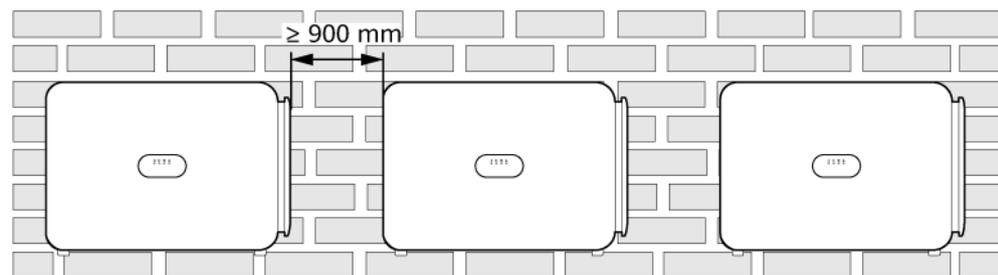
**Figure 4-4 Triangle installation mode (recommended)**
