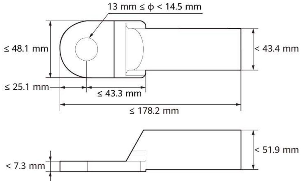
Figure 5-6 Cable connection
