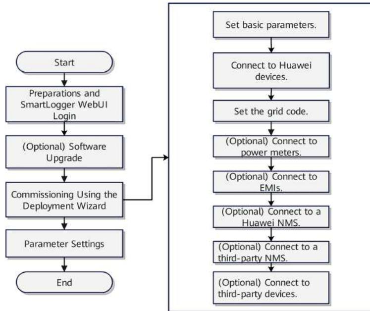
**Figure 7-2** Commissioning process on the FusionSolar app
