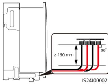
**Figure 5-16** Connecting DC input power cables (AVIC JONHON)
