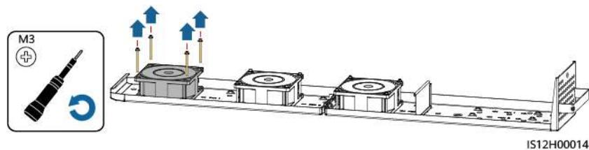
**Step 6** Install a new fan (FAN 1 is used as an example).
