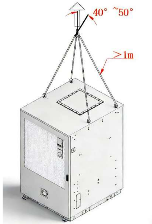
Figure 4-1 Lifting Installation Diagram
