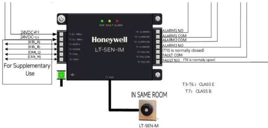
Figure 7-4 Flammable Gas Detector Wiring Diagram
