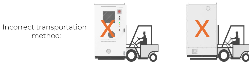
Figure 4-2 Diagram of Forklift Transportation
