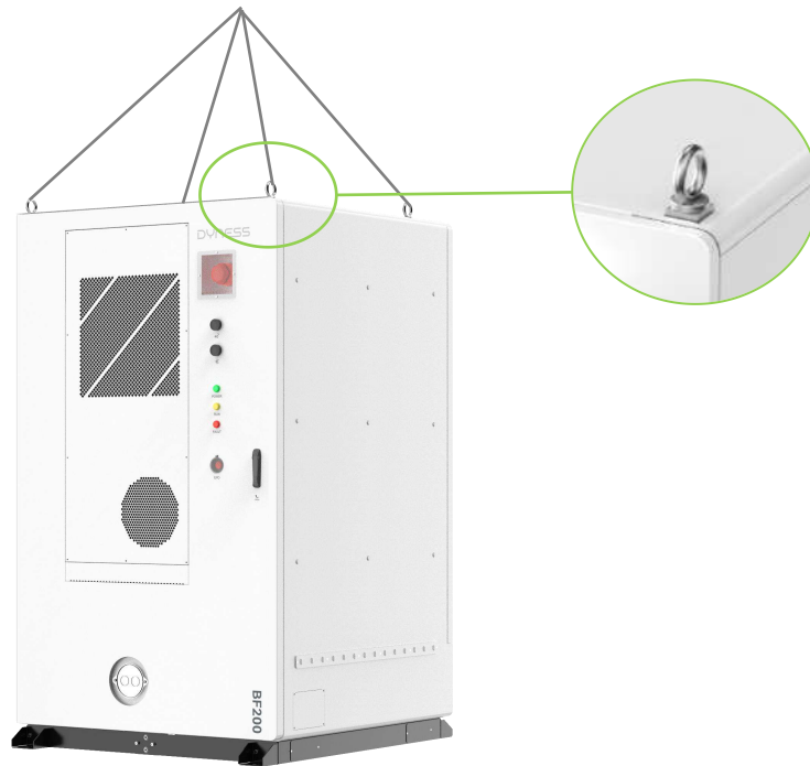
Figure 4-1 Hoisting and Transportation Schematic Diagram
