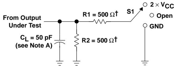
† When  $V_{CC} = 1.5\text{ V}$ ,  $R1 = R2 = 1\text{ k}\Omega$
