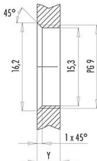
Installation direction: o-ring sits on chamfer.
