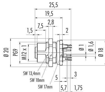
Thickness of PCB: 1,6 mm
