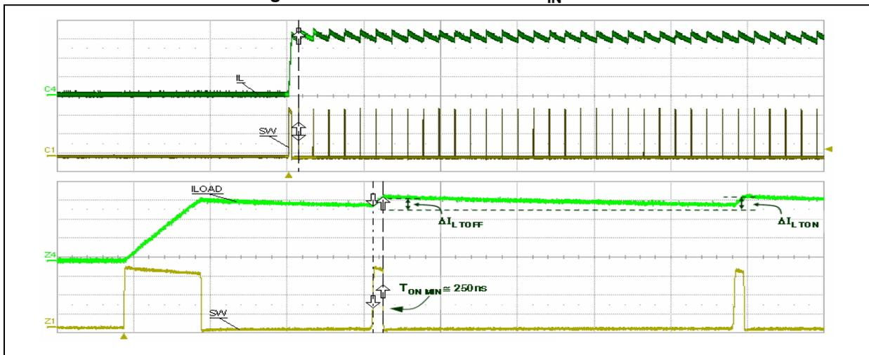
Figure 17. Short-circuit current  $V_{IN} = 36\text{ V}$
