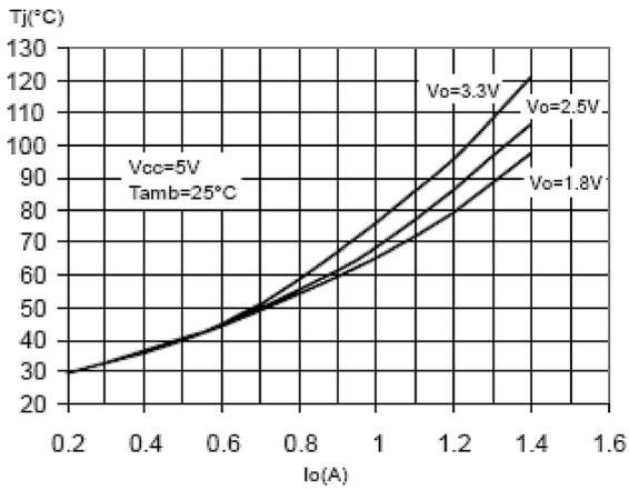
**Figure 34. Junction temperature vs. output current -  $V_{IN} = 12\text{ V}$**
