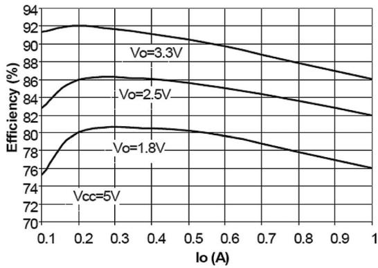
**Figure 36. Efficiency vs. output current -  $V_{IN} = 12\text{ V}$**
