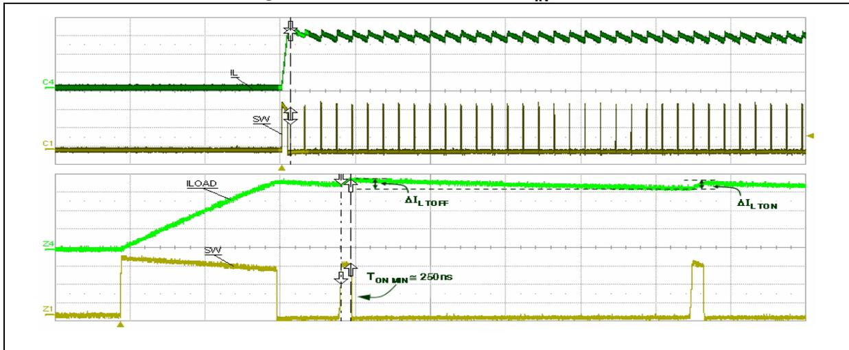
**Figure 16. Short-circuit current  $V_{IN} = 24\text{ V}$**
