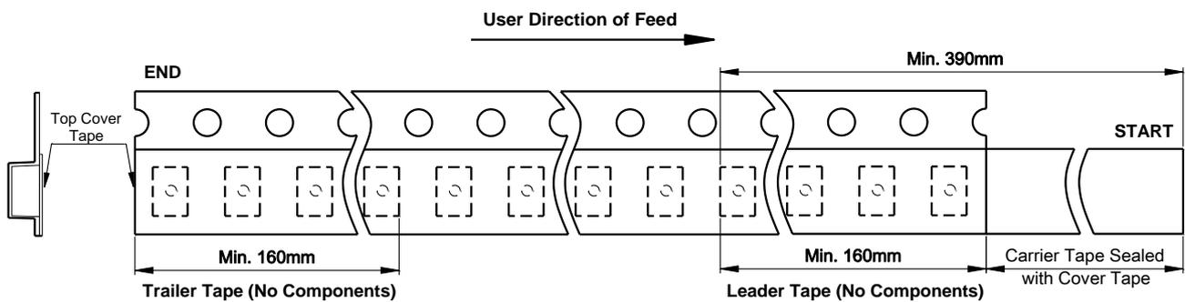
**Note:** There shall be a leader of at least 230mm which may consist of carrier tape and/or cover tape or a start tape followed by at least 160mm of empty carrier tape sealed with cover tape.
