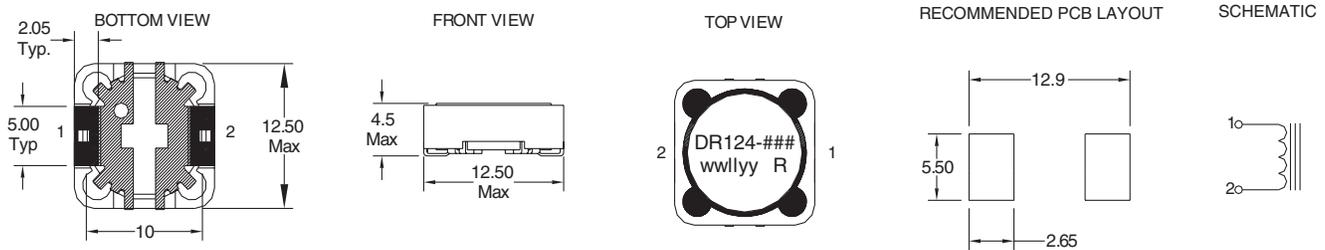
Dimensions are in millimeters.
