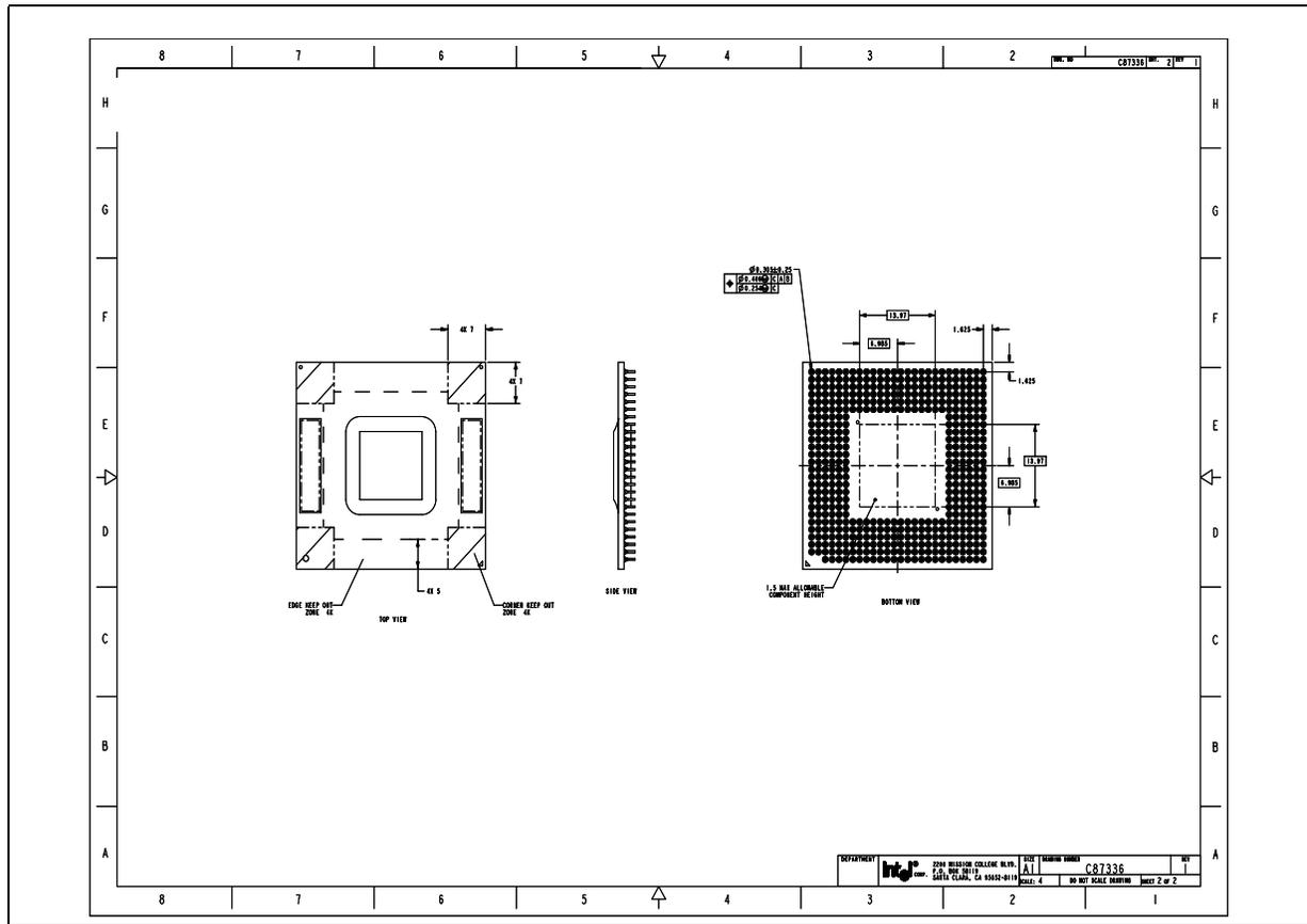
Figure 7. Micro-FCBGA Processor Package Drawing (Sheet 1 of 2)
